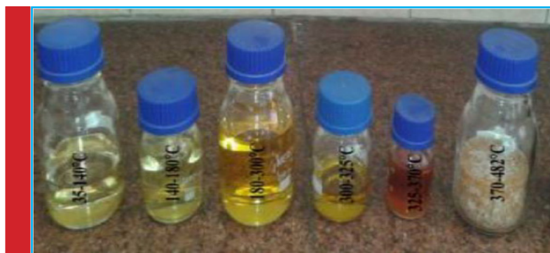
FIGURE 2. Different distillates of biocrude oil
