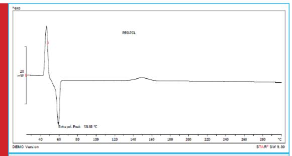
FIGURE 2. The DSC Spectrum of Mpeg-PCL copolymer, it appears in the peak temperature range at 40.3 °C, which can be attributed to the crystallization temperature of PEG.
