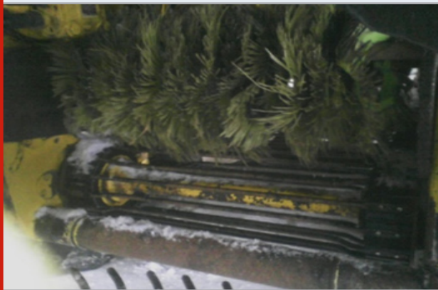
Figure 1: Receiving rod conveyor of the ROPA Euro Tiger combine with installed brush drums
