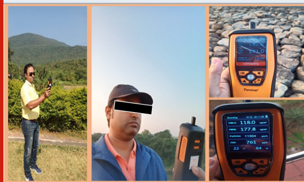
Figure 4: Ambient air quality of Baranti was measured at different spots through Temtop M2000C Air Quality Monitor
