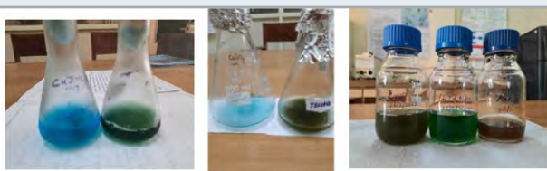
Figure 1: Visual confirmation of Bimetallic Cu-Zn nanoparticles from leaf extracts of Terminalia (a) , Tecoma (b) and c) Solanum
