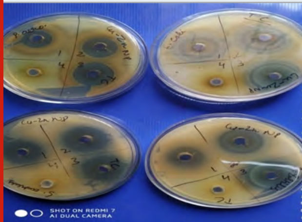
Figure 2: Zones of inhibition using Bimetallic Cu-Zn nanoparticles from Harad leaf plant extracts tested against four pathogens. a) P. aeruginosa b) E. coli . c) S. aureus d) B. subtilis .
