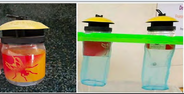
Figure 2: The final flight trap to implement this experiment with high efficiency: the bottom of the traps was removed, and a cloth basket was inserted to collect samples.
