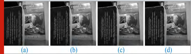
Figure 4: (Book): a. Original Image; b, c. Multifocus input images; d. Proposed fusion.
