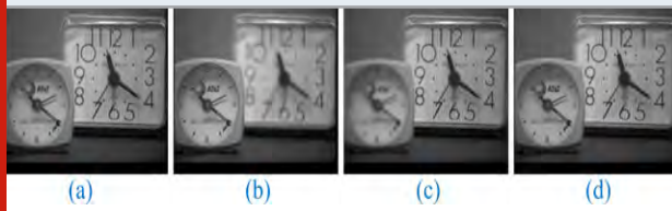
Figure 2: (Clock): a. Original Image; b, c. Multifocus input images; d. Proposed fusion.
