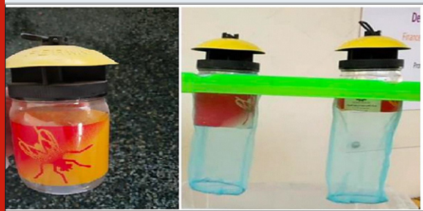
Figure 2: The final flight trap to implement this experiment with high efficiency: the bottom of the traps was removed, and a cloth basket was inserted to collect samples.
