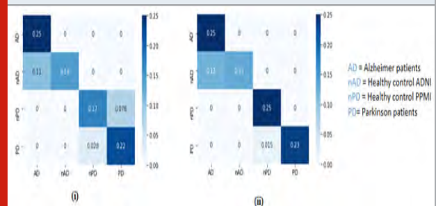
Figure 3: Confusion matrices of the proposed system based on VGG19 (i) with 70/30 validation split; (ii) with 80/20 validation split
