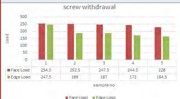
Figure 9: Screw Withdrawal Strength of the board samples
