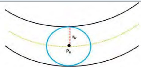
Figure 5: Circular area: In (blue) color is the wheel defining the circular area around center pixel P_0 , r_k is the radius of the wheel.
