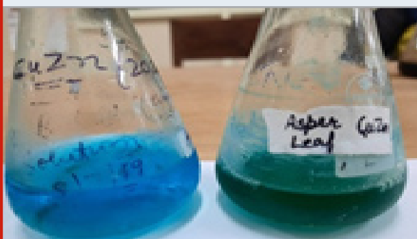
Figure 6: Bimetallic Cu-Zn nanoparticles using plant leaves showing green colored solution in comparison to Cu-Zn solution
