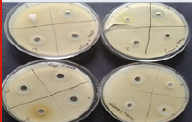
Figure 5: Mono metallic - Zn nanoparticles synthesized using leaf root, stem and thorns of Achyranthes aspera at three different volumes against S. aureus .
