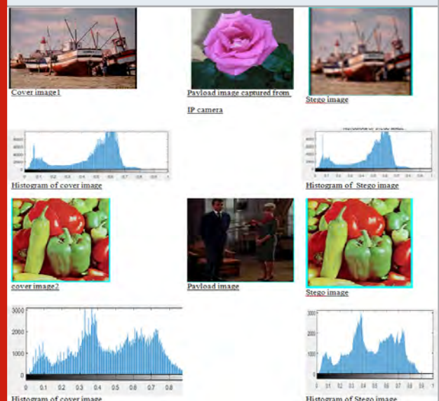
Figure 7: Experimental Results of the proposed method for color images
