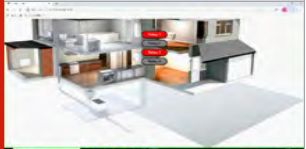
Figure 4.5: Fan and load is controlled by the relay button 1&3 at a time from web page
