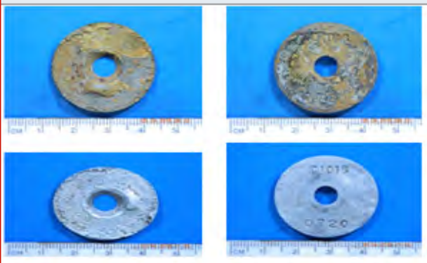
Figure 8: Coupons of wet gas
