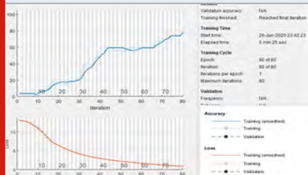
Figure 5: CNN training accuracy and loss graphs.
