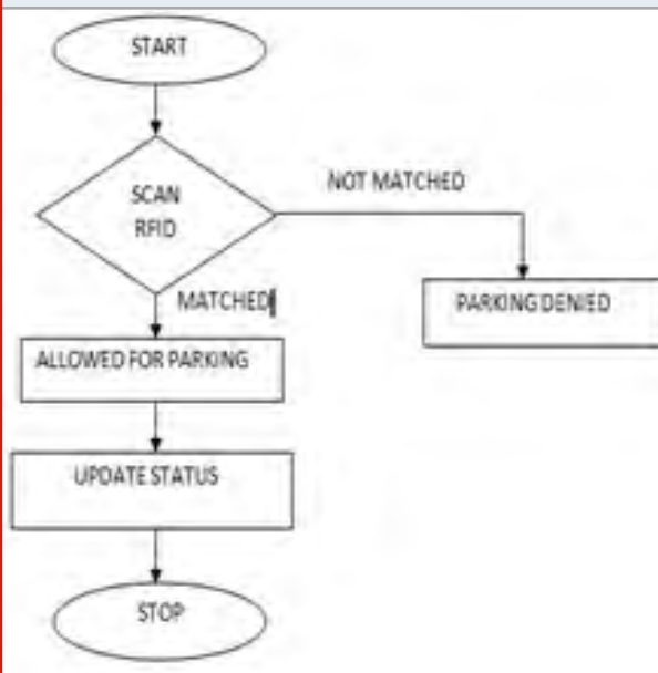
Figure 2: Flowchart for Vehicle Entry
