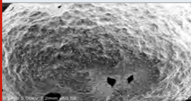
Figure 27: SEM image of Sodium alginate beads before treatment (1mm)
