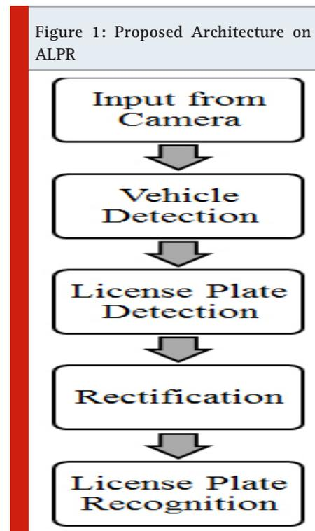
**Vehicle Detection:** The study used GAN algorithm for the license plate detection in vehicles, since the vehicle is one of the underlying artefacts in many traditional detection algorithms. We found the following problems when selecting an object detection algorithm: The algorithm, for one, necessitates a high level of accuracy. Second, the algorithm necessitates a fast measurement speed, so
