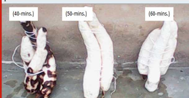
Figure 7: Effect of 30% lye-concentration on whole cassava roots after hand brush-scrubbing of digested peel at 32 °C
