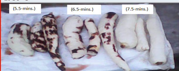
Figure 8: Effect of 35% lye-concentration on whole cassava root after hand brush-scrubbing of digested peel at 50 °C
