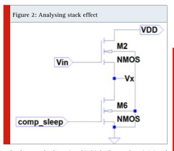
In sleep mode sleep signal is high. Comp\_sleep is '0' and when Vin='0'. From Low power methodology manual: for system-on-chip design and Scaling of stack effect and its application for leakage reduction proposed by (Flynn et al., 2007; Narendra et al., 2001) Modified the standard leakage power equation by replacing ex component by 10x component.
