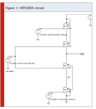
The Multi Threshold CMOS circuit will reduce the static power dissipation by reducing leakage power in sub threshold region. Because Pull down is not directly connected to the ground but through the virtual ground. It has the node potential Vx greater than ground potential.
