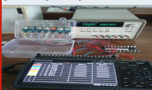
Figure 1: Experimental set up for measuring volatiles of green chilli using sensor array
