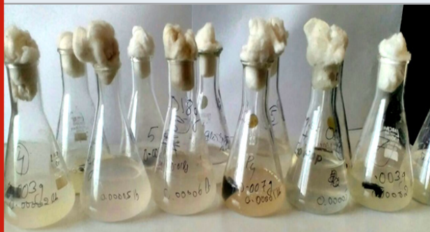
Figure 2: Microbial degradation of plastic in liquid medium after 15 days of inoculation
