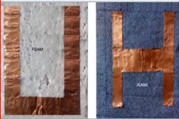
Figure 2: Fabricated antenna geometry (a) middle & (b) bottom view with foam substrate
