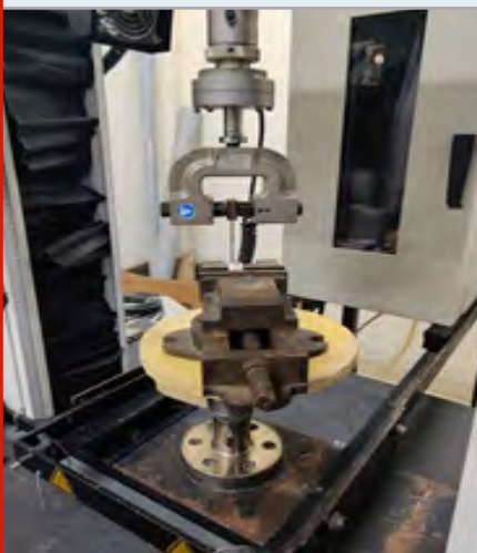
Figure 5: The brackets held at their crossheads by the instron testing machine just prior to debonding.
