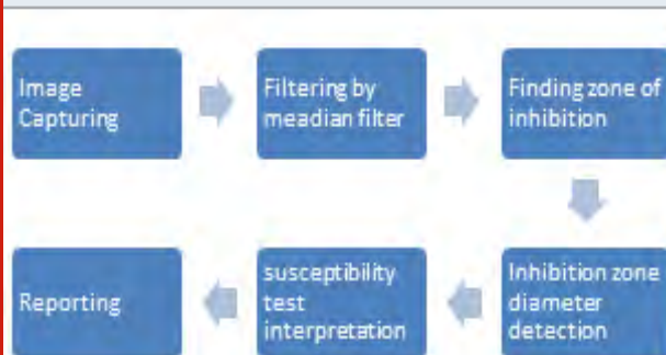
Figure 1: AST Processing Diagram with Image Processing
