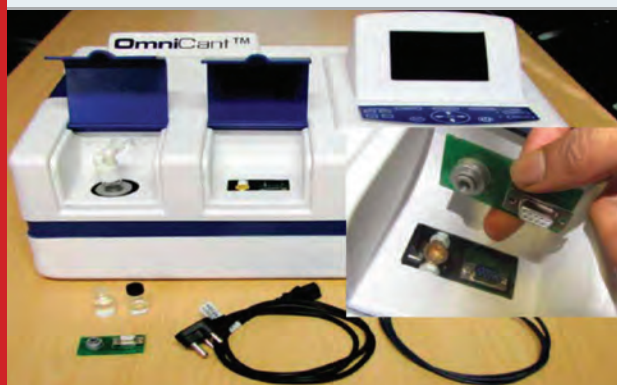
Figure 3: Omnicant setup used in experimentation
