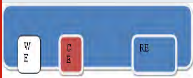
Figure 1: Schematic of biosensor with 3 electrodes
