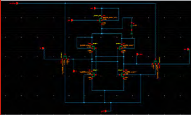
Figure 7: schematic of proposed 7T SRAM using power gating during write mode
