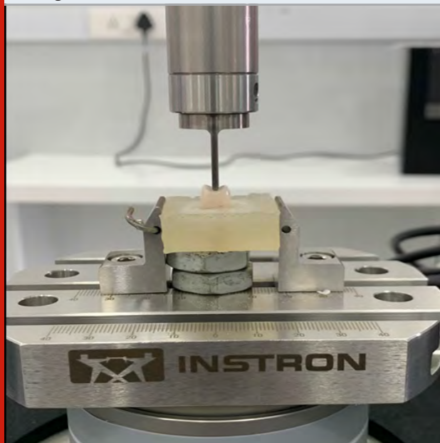
Figure 2: Showing a sample from Group 2 (a new unrestored Nissin typodont mandibular first premolar) mounted parallel to the long axis of the tooth and ready to be tested for its fracture strength in an Instron universal testing machine.
