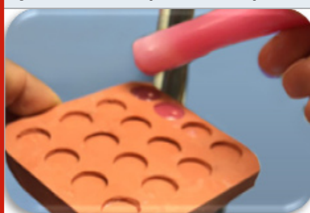
Figure 1: The mold filled up with melted base plate wax.
