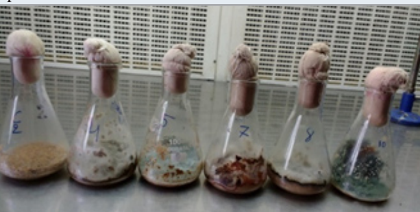
Figure 2B: Solid State Fermentation for cellulase production
