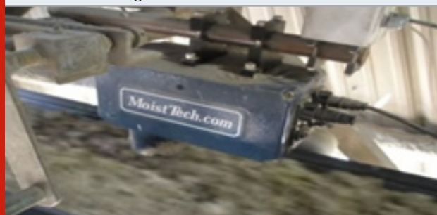
Figure 2: Existing method of bagasse moisture monitoring and control using NIR Sensor
