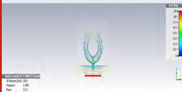
Figure 7: 2.70 GHz Surface current
