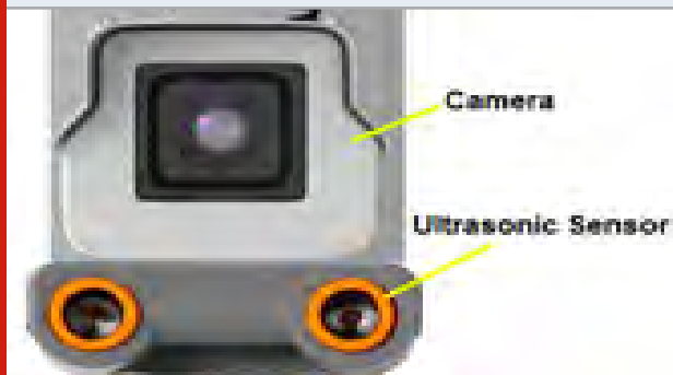
Figure 5 (a): Camera with Ultrasonic Sensor
