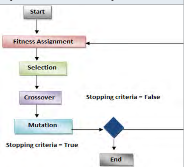
Figure 1: Flowchart for Genetic Algorithm
