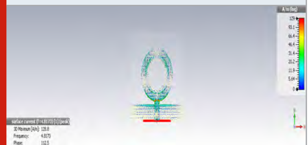
Figure 10: Surface current at 4.81 GHz
