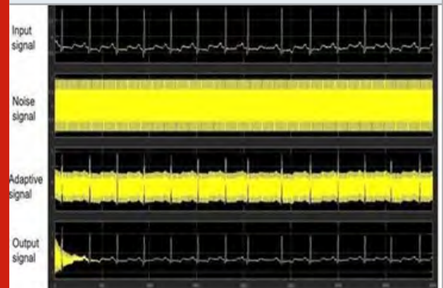
Figure 8: Simulation output of 4 tap lattice LMS filter structure
