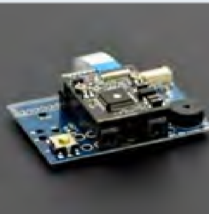
Figure 4: Barcode scanner with CCD camera
