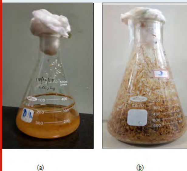
Figure 3: (a) (b) - Laccase production using submerged fermentation and solid state fermentation
