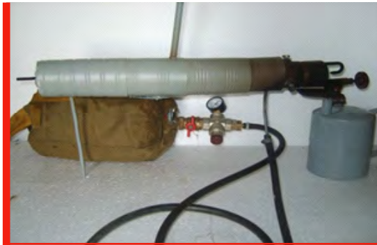
Fig. 1: Autonomous steam generator.
