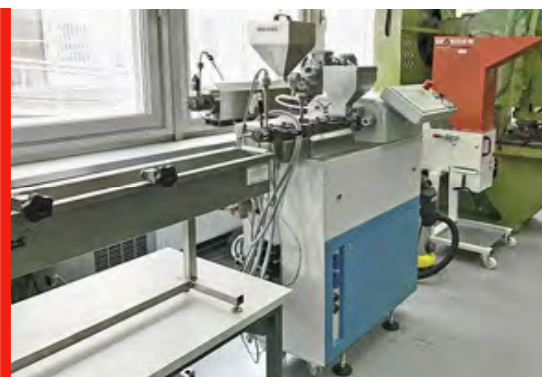
Fig. 1: Laboratory twin screw extruder
