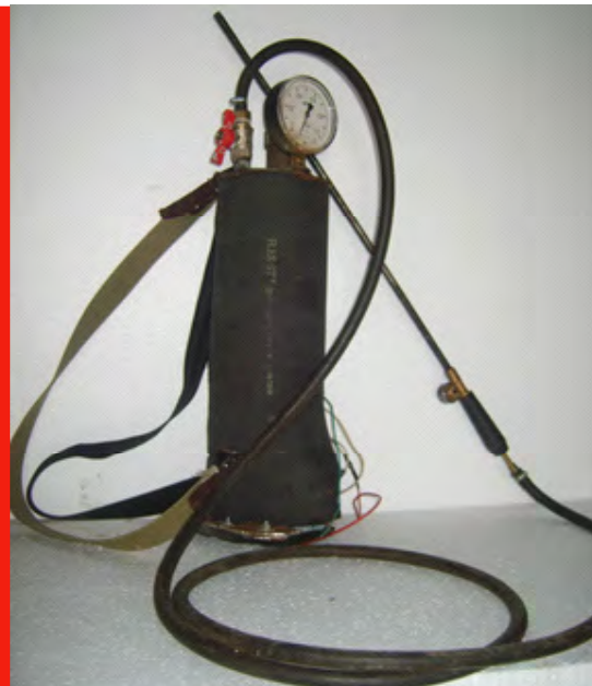
Fig. 2: Electric steam generator.
