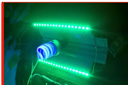
Fig. 1: Prototype model of the irradiating device complete with the powered UV lamp and LED strip.
