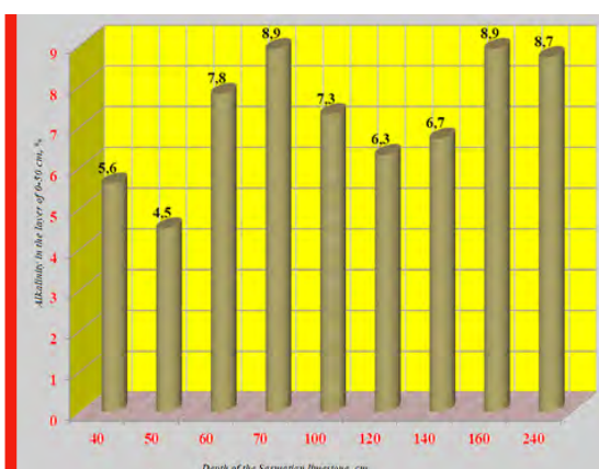
Fig. 2: Histogram of changes in the soil alkalinity, depending on the depth of the Sarmatian limestone
