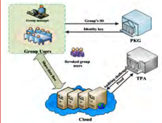
Figure 2. The system overview of TPA
