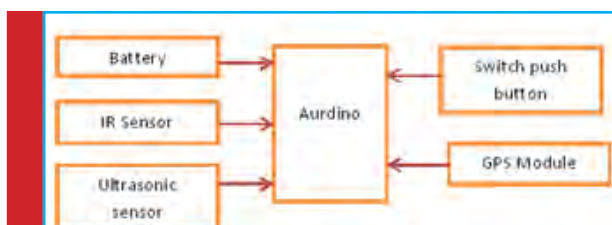
Figure 1. Block diagram of blind stick using arduino
