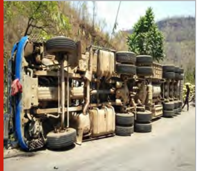
Figure 3: Collapse of over load vehicle due to unbalance
