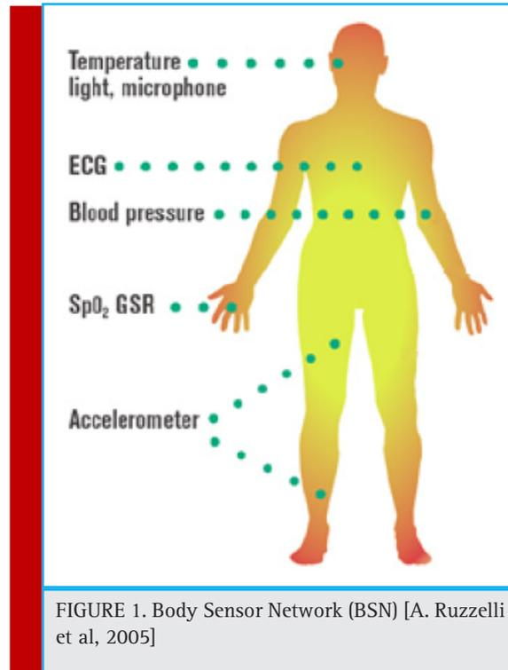
FIGURE 1. Body Sensor Network (BSN) [A. Ruzzelli et al, 2005]
