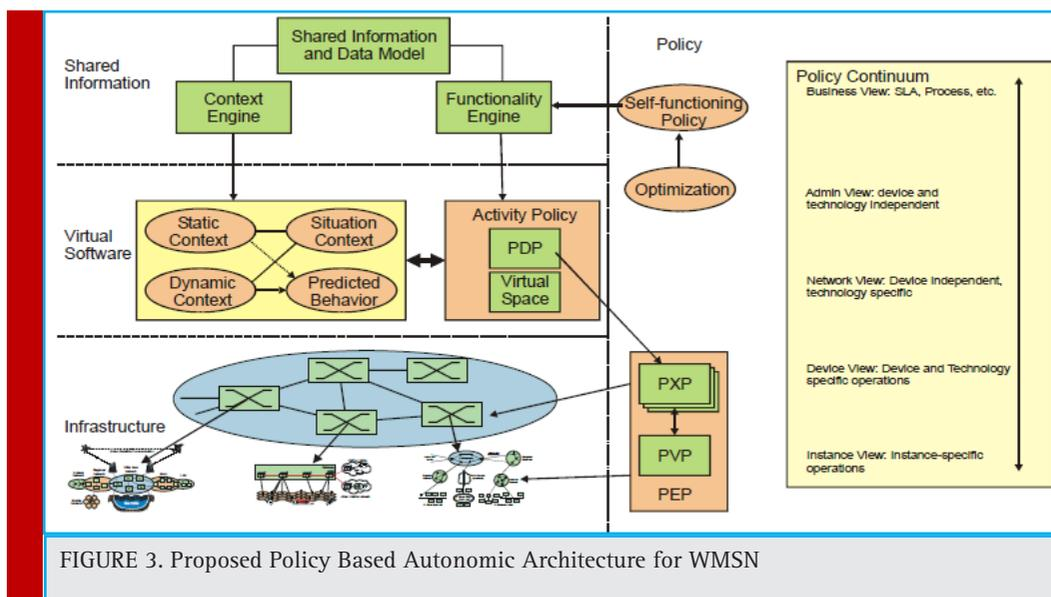
FIGURE 3. Proposed Policy Based Autonomic Architecture for WMSN
