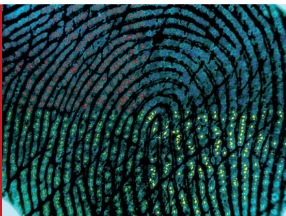
FIGURE 3. A view of sweat gland pores in the left thumb using MIP4.2 Full software and a microscope (Dino-Lite-Plus AM313) with 65 \times magnification; the pores were classified into four parts identified by red, blue, green, and yellow colors.
