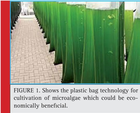
FIGURE 1. Shows the plastic bag technology for cultivation of microalgae which could be economically beneficial.
